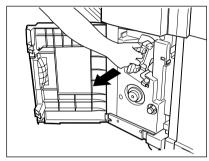
**9** Pull out the grip of the saddle staple holder ① toward you and turn it ② 90° clockwise in the direction of the arrow.
